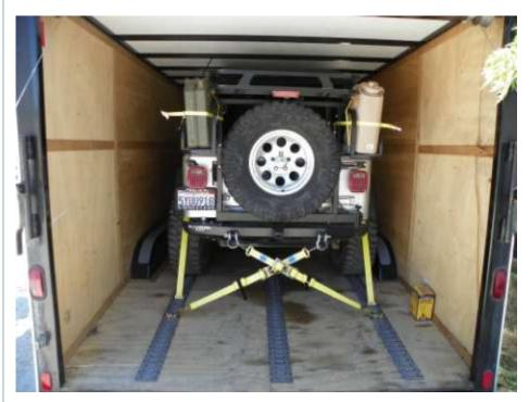
nally from the bumper D-rings to an eTrack D-ring on the opposite tire line, two in the front and two in the rear (we were worried about hitting a bump and the jeep bouncing off the ceiling). Strapping the tires down took all of the play out of the sidewalls and, believe it or not, the Jeep would not move! No sway, no bounce, nothing! As a result the diagonals were a little over kill (someone asked if I was a loadmaster securing a Abrams tank).
