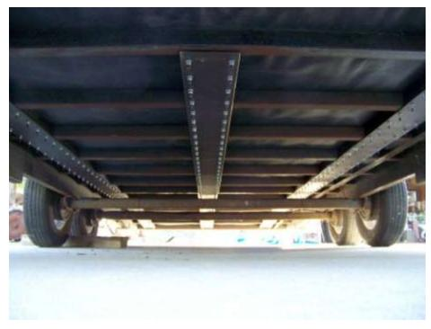
the small box beams thru the flooring to hold them in place. The rubber coated plywood laminate that
