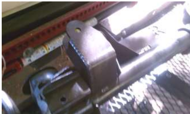
old track bar mounting hole to center tie-rod.
